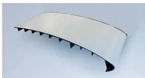
Figure 1. Clean Sky test object representing NLF integrated wing panel.
