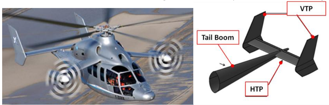
Figure 1. Structural components of the LifeRCraft tail unit***
