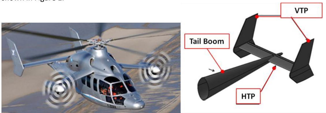
Figure 1. Structural components of the LifeRCraft tail unit ***
