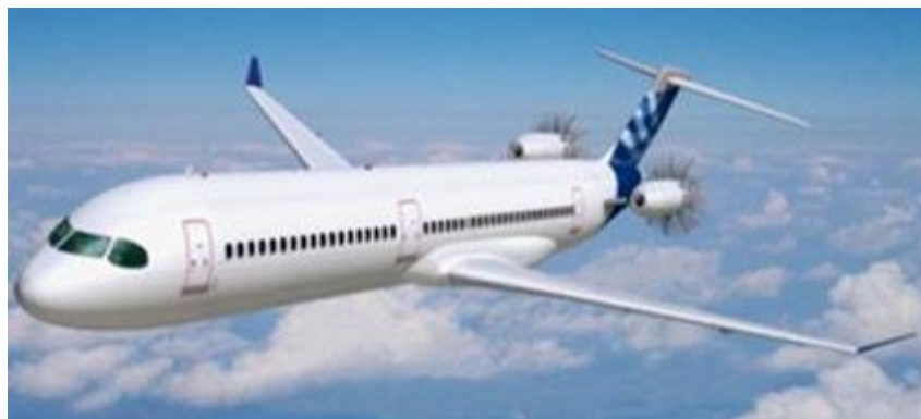
Figure 2. R&T concept study with rear mounted open rotor engines
